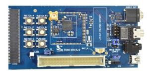
This board features the latest CSR BlueCore® CSR8605 QFN Bluetooth audio solution. It interfaces with mono headphones and has flexible LED and push-button assignments. Battery current measurements can be performed, and a PIO header allows for connection of further application hardware, such as displays.
